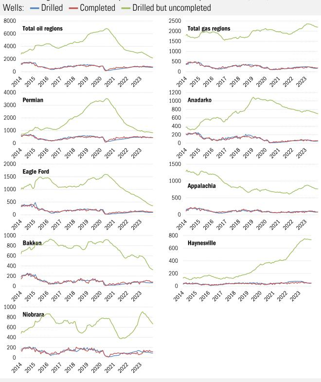
Low fracking fruit: the inventory of drilled but uncompleted wells (DUC)
